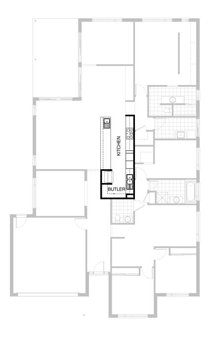
Provide Galley-style Kitchen upgrade option with Butler's Pantry in lieu of WIP, including: additional benchtop and tiled splashback, relocated Ref. space with 920mm laminate open shelf, 1No. 900mm retractable rangehood,
