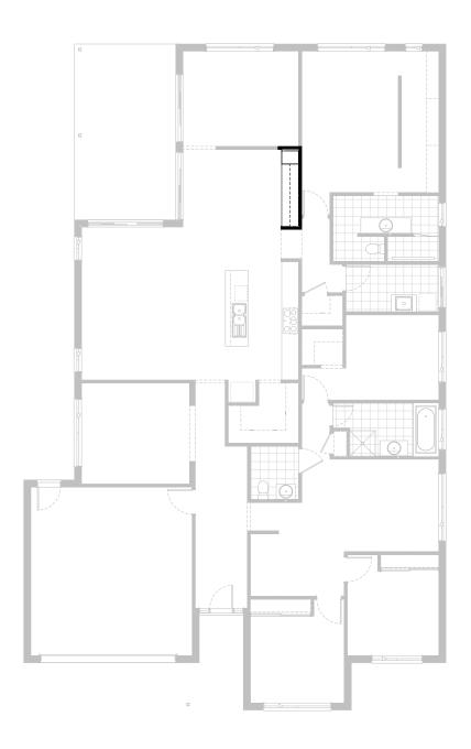
Provide built-in joinery option to create Study Nook near Meals area, including: 600mm deep 32mm thick laminate desktop, 1No. 450mm laminate linen unit, 1No. 450mm drawer unit below desk, 2No. 300mm deep 60mm thick open shelves. Remove bulkhead over (unless ceiling height is raised to 2740mm)
