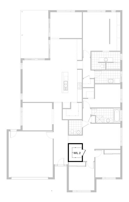
Provide Walk-in Linen option in lieu of Study, including: additional stud and plaster walls, 3No. 450mm shelving, 820mm hinged door.
