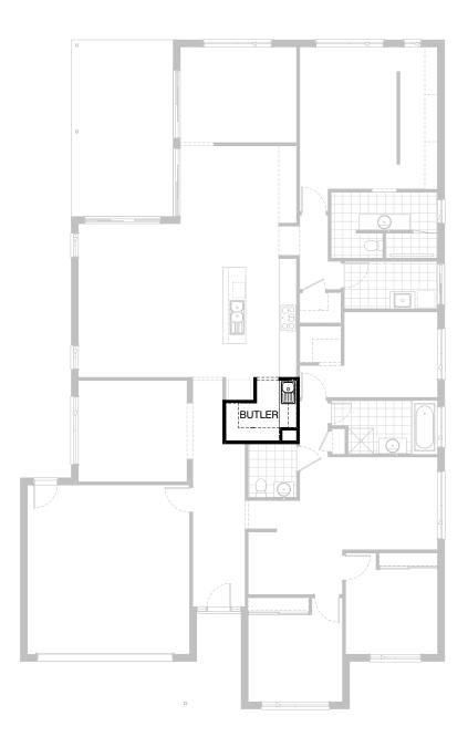
Provide Kitchen upgrade option with Butler's Pantry in lieu of WIP, including: additional laminate benchtop, 2No. 800mm base cupboards, 2No. 300mm deep 60mm thick open shelves, over Butler's sink. Provide plaster-lined void and remove 1No. 450mm shelving.
