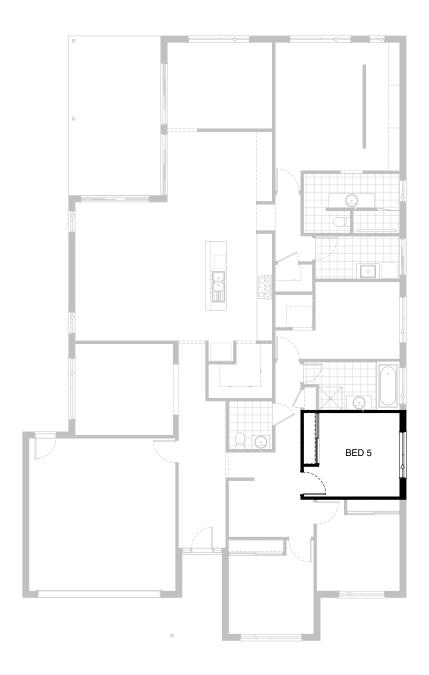
Provide Bedroom 5 option in lieu of Activity room, including: built-in Robe with 450mm shelf and hanging rail with full-width sliding doors, 870mm hinged door in lieu of opening, 1200mm x 1810mm aluminium sliding window in lieu of standard.
