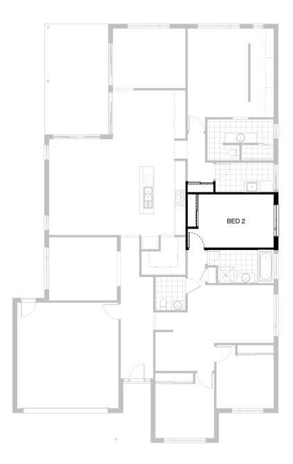
Provide standard built-in Robe and Linen cupboard with sliding doors in lieu of Walk-in Robe and Walk-in Linen. Option increases the size of Bed 2 by 970mm.
