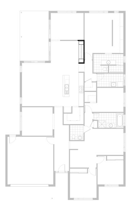
Provide built-in joinery option to Nook near Meals area, including: 600mm deep 32mm thick laminate benchtop, 2No. 900mm base cupboards with drawers, 2No. 400mm laminate linen unit, 2No. 300mm deep 60mm thick open shelves. Remove bulkhead over (unless ceiling height is raised to 2740mm)
