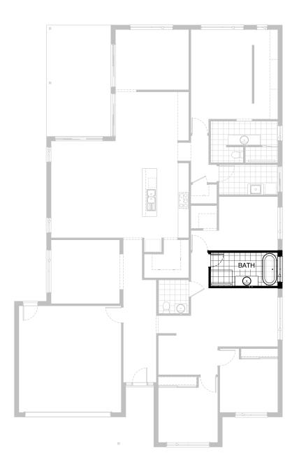
Provide Bathroom upgrade option, including: 1780mm freestanding bath, 1200mm x 900mm tiled shower base with grate drain, 1282mm vanity with single basin. Remove Linen cupboard from Passage.
