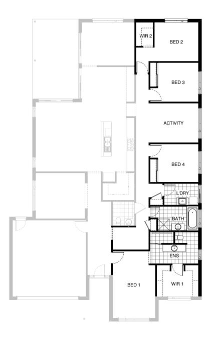
Provide floor plan option that moves Bed 1 to the front of the home as shown.
