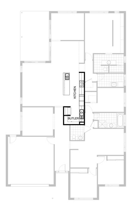
Provide Kitchen upgrade option with Butler's Pantry in lieu of WIP, including: additional benchtop and tiled splashback, relocated Ref. space with 920mm
