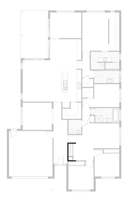
Provide built-in joinery option to Study Nook near Activity, including: 600mm deep 32mm thick laminate desktop, 1No. 450mm laminate linen unit, 1No. 450mm drawer unit below desk, 2No. 300mm deep 60mm thick open shelves.
