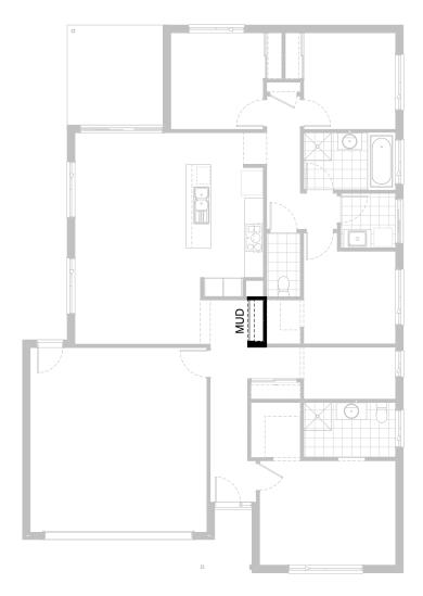
Provide built-in joinery option to Nook to create Mud room, including: 450mm deep 32mm thick laminate benchtop, 2No. 600mm T.V drawer units, 2No. 300mm deep 60mm thick open shelves over. Provide 180mm nib wall with bulkhead over.
