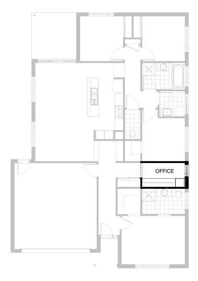
Provide built-in joinery to Office, including: 600mm deep 32mm thick laminate desk, 1No. 450mm drawer unit under desk, 1No. 600mm laminated cupboard, 2No. 300mm deep 60mm thick open shelves.
