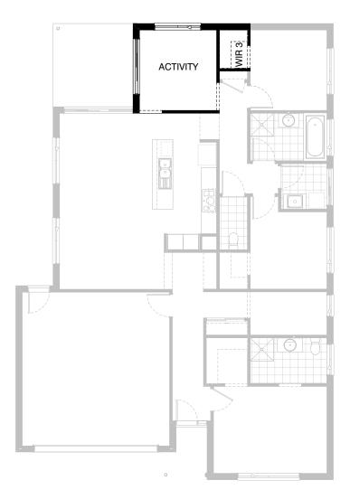
Provide Activity in lieu of Bed 4, including: additional 1No. 2110mm x 2170mm aluminium sliding door, remove built-in robe and 1No. 870mm hinged door and provide 2No. bulkhead openings. Provide walk-in robe to Bed 3 in lieu of standard built-in Robe.
